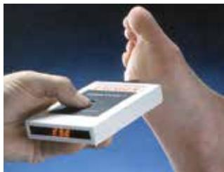
The DermaTemp is a high precision hand-held infrared thermographic scanner designed to detect the subtle skin temperature variations caused by underlying perfusion variations. These instruments feature a patented automatic emissivity compensation system for absolute accuracy regardless of skin type or color. In those applications where cross-contamination is an issue, the use of disposable wraps or sheaths allows even moist or wet tissue to be measured with precision accuracy.
